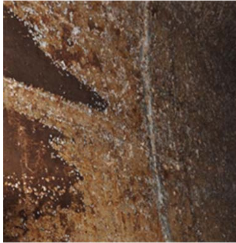
Figure 5.2 Evidence of biofouling and a resultant abrasive surface on the draft tube of a La Rance turbine (photo: Nicola Teague)
